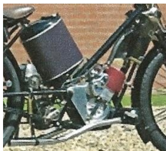
Fig. 2. 1913 Scott 2-cylinder. Water-cooled cylinders; air-cooled heads (DASO 289).
