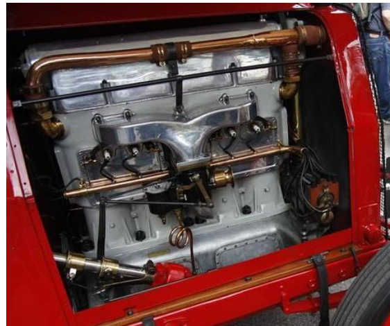
Fig. 2 PEP340 1912 Daimler DF80 IL6 105 mm/140 = 0.75 7,274 cc 100 HP @ 2,000 RPM As tested by Rolls-Royce in 1914; see DASO1097. Daimler entry for 1912 Kaiserpreis aeroengine competition, later fitted with flywheel and clutch for use in the 1913 Mercedes racing car.
