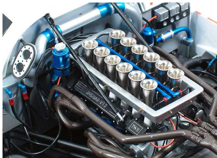
Fig. 32 PEP 261 1988 Jaguar TWR Le Mans 60V12 94 mm/84 = 1.119 6,995 cc 826 HP @ 7,500 RPM
