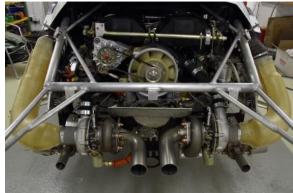
Fig. 31 PEP 351 1978 Porsche 935/71 F6 95.7 mm/74.4 = 1.286 3,211 cc 750 HP @ 8.000 RPM Water-cooled 4v/c heads, air-cooled cyls. As installed in the type 935/78 car "Moby Dick", which reached 228 MPH at the 1978 Le Mans, but only finished 8 th . Teamspeed.com
