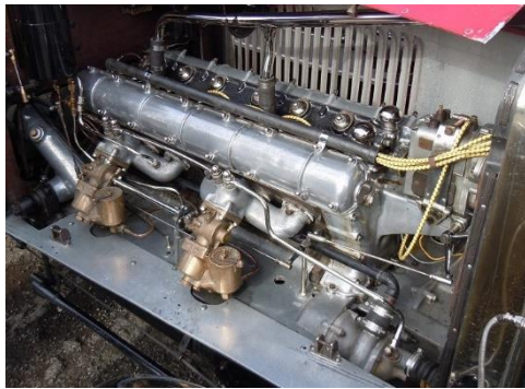
Fig .4 1925 Sunbeam 3 Litre IL6 75 mm/110 = 0.682 2,916 cc 90 HP @ 3,800 RPM
